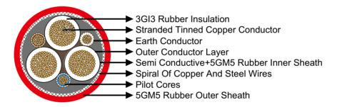
**Conductors:** Flexible stranded tinned copper conductor. **Insulation:** Heat resistant 3GI3 rubber based on EPR.
